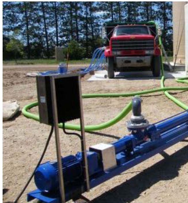
Pump with VFD to the Dewatering!
